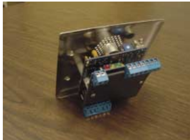
FIGURE 2 Sensitivity Pot, and terminal blocks as described in text
